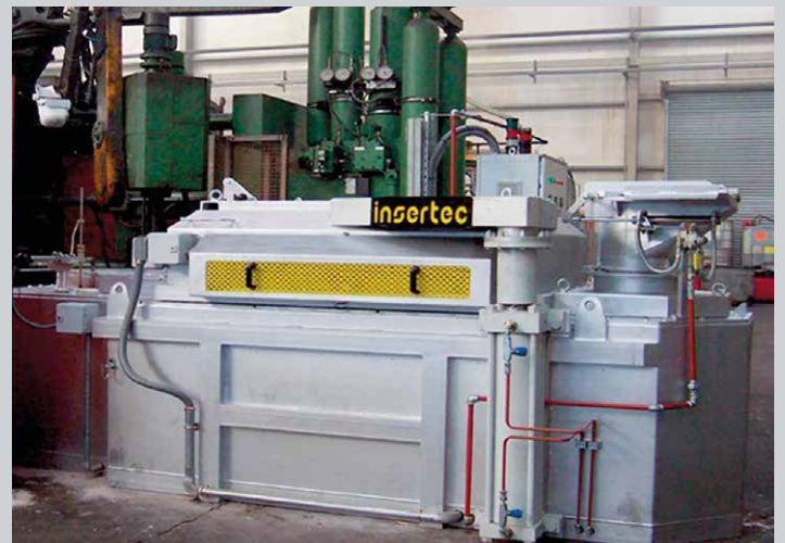
\ Holding furnace Horno mantenedor
