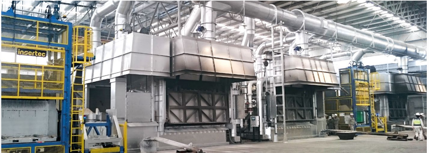
\ 35 Mton stationary sidewell melter.
