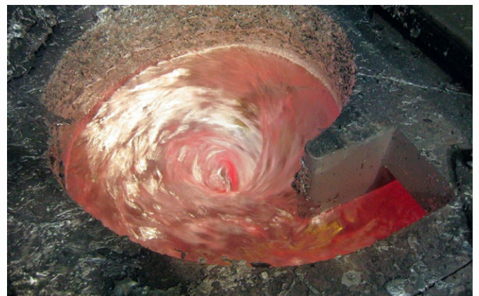
\ Sink vortex with molten metal on recirculation .
